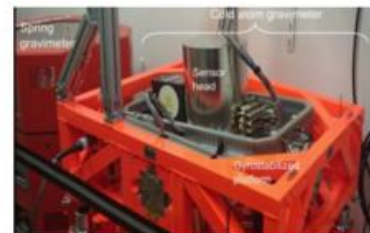
ONERA's embarkable cold atom gravimeter
