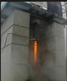
Combustion chamber Hot-fire test (HTP)
