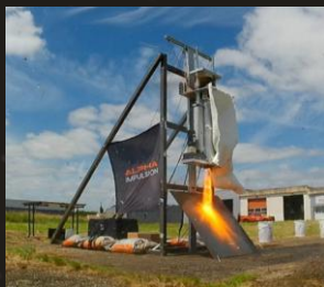
1st ignition autophage Engine (HTP – HDPE)
